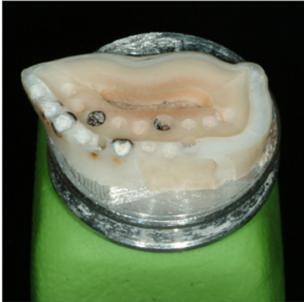
Fig 1 A 3-mm sample fixed on an SEM holder by means of composite resin.
